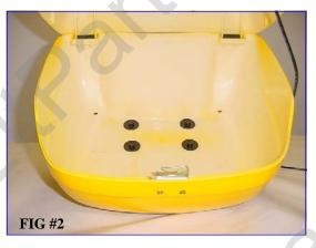
The mounting plate is positioned on the bottom of the luggage box with the smooth side toward the box. The (4) bolts and washers are pushed through the box and plate from inside the box using the holes indicated in Fig #3.
