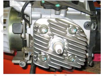
Remove the cylinder head.
