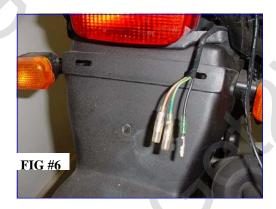
The wires for the LED hookup are located on the rear of the bike around the rear taillight. They may be tucked in under the harness on the left hand side of the unit..
