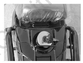
Unscrew two taper screws of the body cover near the footrest board. Remove the body cover.
