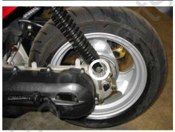
Remove the engine hanger nut.
