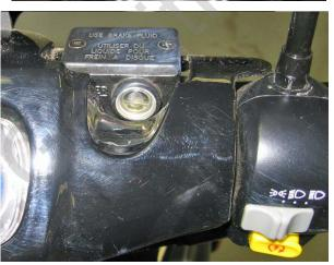
Engage the front brake a few times by pulling the brake lever gently. Then, hold the front brake level all the way in; while holding in, release the bleeder valve on the front caliper to force the air out. Then, lock the valve. Repeat this action until no more air flows out. Torque value: 4 lbf-ft
