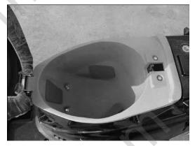
Unscrew the fixing screws between the body cover and middle cover.
