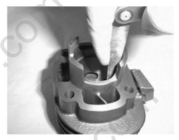
Measure the clearance between the ring and groove.
