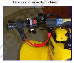
RXL-40E safety tether switch wiring. Red/Black wire female end from the harness to the Red/black wire male end from the switch. White wire male end from harness the white wire female from switch.
