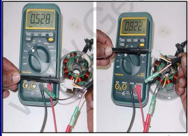
To test the exciter coil, set the multi-meter to a 1k ohms scale. Check the ohms from the white/red wire to the generator case or ground as shown in Figure 2. The reading should be 0.520—0.535 k ohms.
