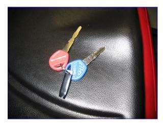
The UK1-90R Rover is equipped with 2 different speed range keys. The blue (shorter) key is restricted to slower RPM and with no adjustment . The red (longer) key is unrestricted with a higher RPM speed range.
