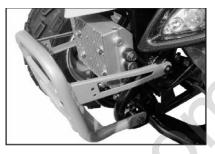
6. Install front bumper using 8x16mm bolts (2), 8x35mm bolts (2)and Front Bumper Collar (2). Torque to 16flb
