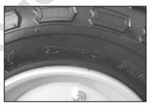
11. Install front and rear wheels. Note rotation arrows on tires when installing.
