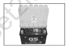
3. Prep battery by adding electrolyte. (About 1 hour for battery to come to full charge. **DO NOT** Put on charger.)
