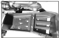
16. Install left footrest & right footrest using 6x18mm button head screw(7), 6x16mm hexagon head bolt (1) and flange Nut (3).
