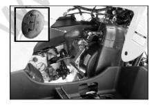
29. Move gear shift shaft into neutral position.
