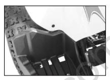
17. Install left footrest & right footrest using 6x23mm button head screw (2) and Flange Nut (2).
