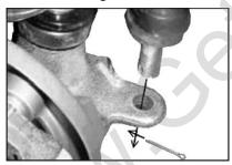
4. Attach tie rod ends using 10mm Lock nut (2). Torque to 25flb and install <sup>3</sup>/<sub>4</sub> cotter keys (2).
