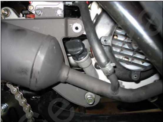
Remove the exhaust pipe
