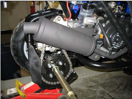
Jack the rear end of the vehicle up, and remove the RH rear tire
