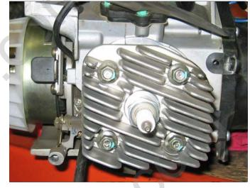
Remove the cylinder head.
