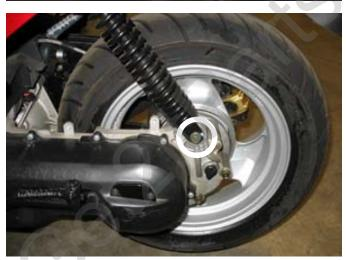
Remove the engine hanger nut.
