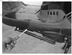
Open the seat. Unscrew four fixing bolts of the helmet box. Remove the helmet box.
