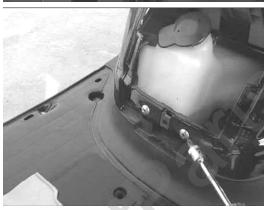
Open and remove the fuel tank cap. Unscrew the two fixing screws of the body cover near the fuel tank cap.
