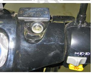
Engage the front brake a few times by pulling the brake lever gently. Then, hold the front brake level all the way in; while holding in, release the bleeder valve on the front caliper to force the air out. Then, lock the valve. Repeat this action until no more air flows out. Torque value: 4 lbf-ft
