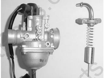
Remove the needle clip retainer, the jet needle, and needle clip. Inspect the throttle valve and jet needle surface for wear, scratches, or dirt.
