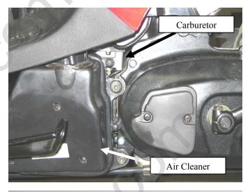
Remove the carburetor cap. Remove the throttle cable from the throttle valve while depressing the throttle valve spring.
