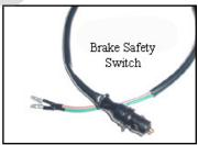
Check left hand brake switch for proper operation. Does brake light remain on?
