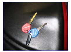
The UK1-90R Rover is equipped with 2 different speed range keys. The blue (shorter) key is restricted to slower rpm's, and with no adjustment on the CDI revlimiter. The red (longer) key is unrestricted and the speed can be increased or decreased with the 1-4 adjustments on the CDI box. Check the chart below for the speed ratings.
