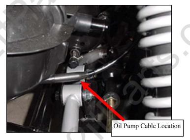
To reduce the oil flow you must lengthen the cable by loosening the lock nut and turning the adjusting nut counter clockwise then retighten the locking nut. To increase the oil flow you would shorten the cable by turning the adjusting nut clockwise.
