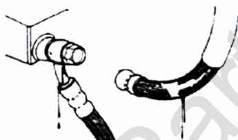
(leak, damaged, looseness of brake line)
